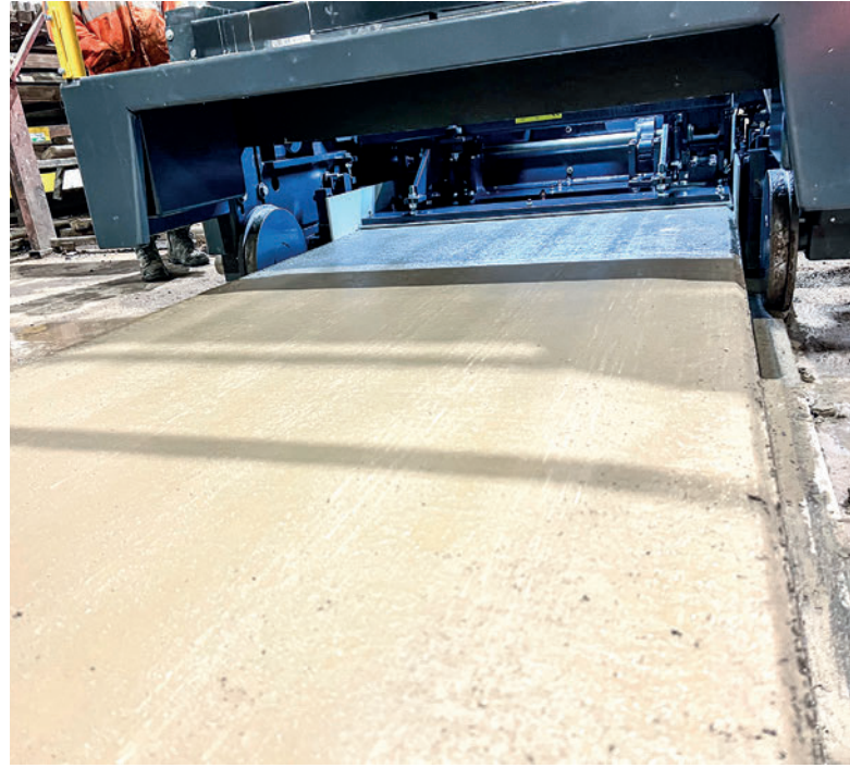
The concrete is directly compressed into the production beds and remains behind the machine to cure.
